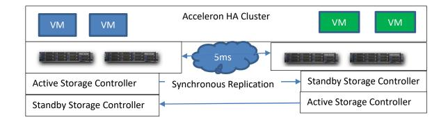
The Acceleron HCI platform supports Metro Availability in conjunction with other data management features, including compression, deduplication, and tiering. Metro Availability also allows you to enable compression for the synchronous replication traffic between the Acceleron clusters. When you configure the remote site, enabling replication traffic compression reduces the total bandwidth required to maintain the synchronous relationship
